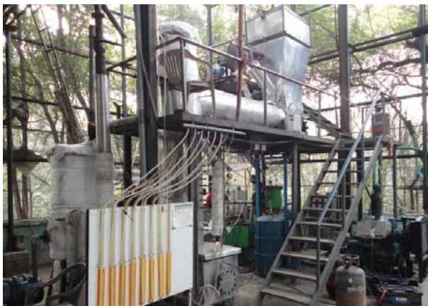
Two-stage gasifier system
