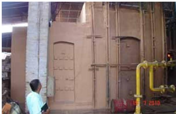
Regenerator in a tank furnace unit
