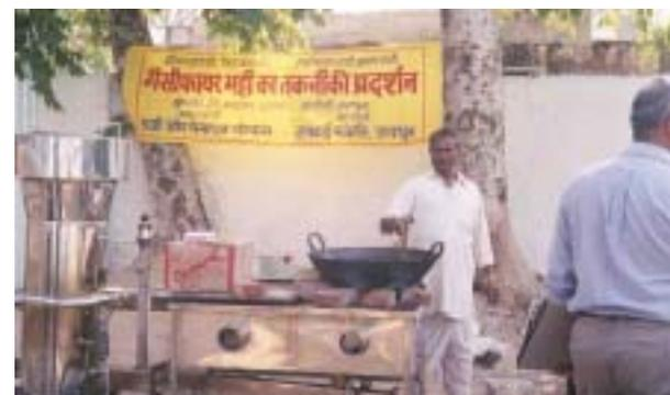
Biomass gasifier for namkeen making
