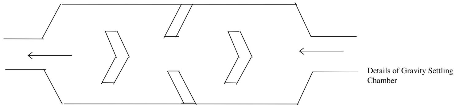
Figure 3. Schematic diagram showing placement of gravity settling chambers in CBRI fixed chimney kiln.
