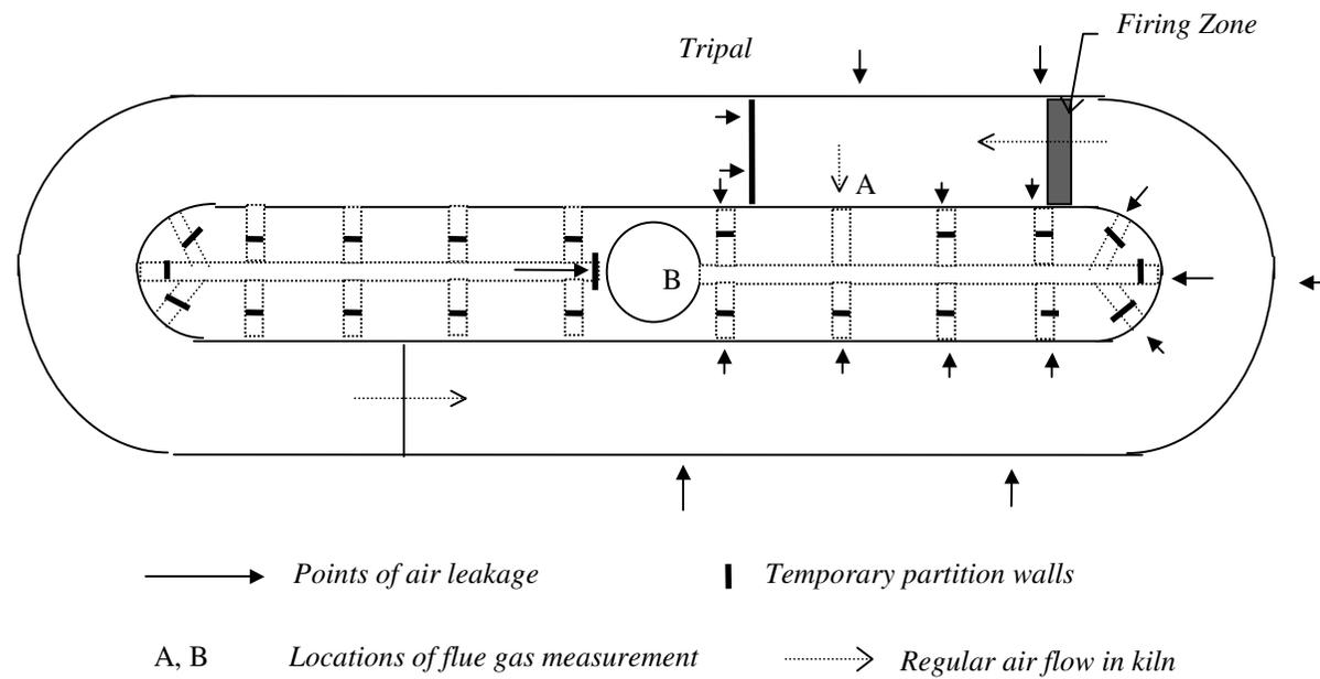
Figure 5. Probable locations of air leakage
