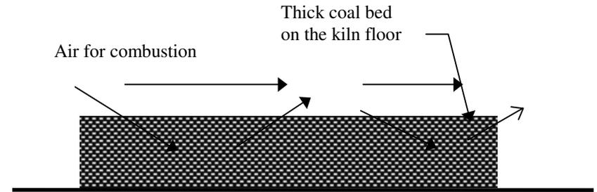
Figure 7. Operating practice - heavy charging of coal, air is not able to diffuse into thick coal bed
