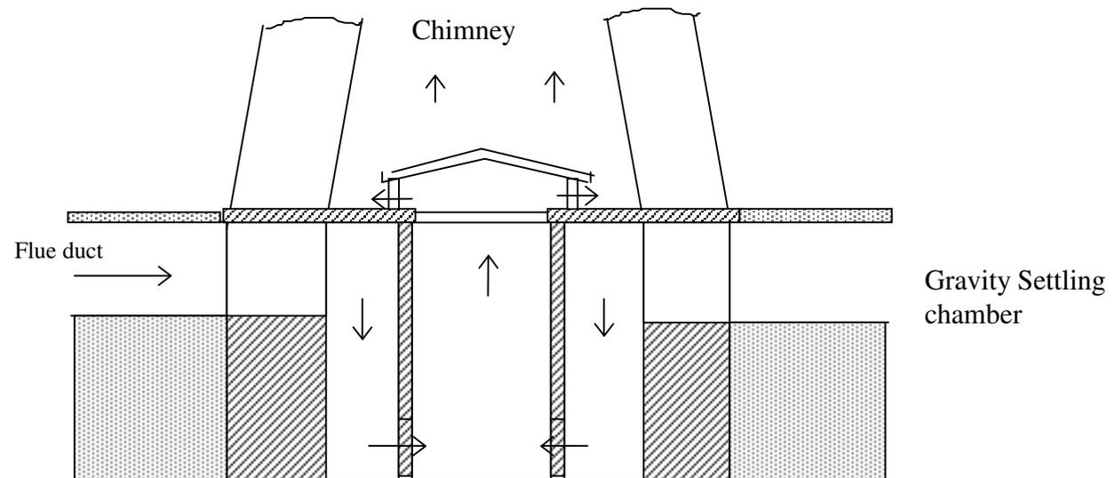
Figure 2. Schematic Plan and details of gravity settling chamber of Priya/PSCST fixed chimney kiln
