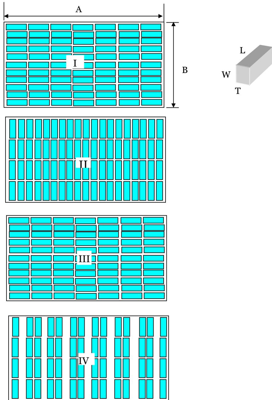
**Figure 3.2** Layer by layer brick arrangement in a batch
