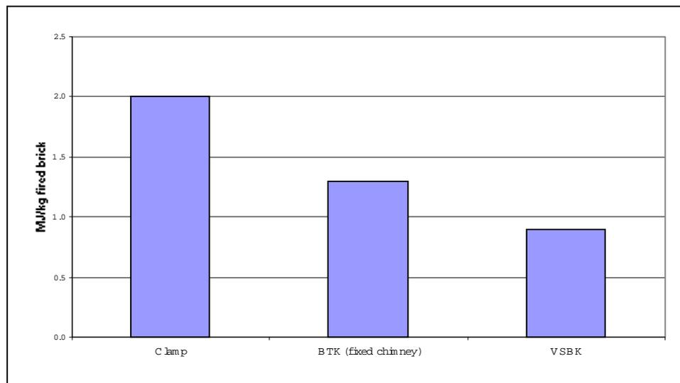
**Figure 4.1** Specific energy consumption of brick kiln technologies
