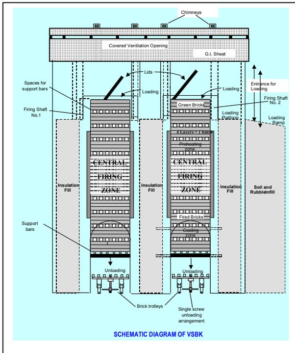
The inside surface of the shaft is generally lined with refractory bricks which ensures long life of furnace wall and minimum maintenance. The gap between the shaft wall and outer kiln wall is filled with insulating materials - clay and rice husk, etc. For monitoring the position of fire and the temperature, peepholes are provided.
