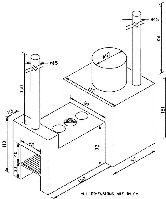
Fig. 2. Traditional cottage basin oven with two chimneys and single row of cooking basins.
