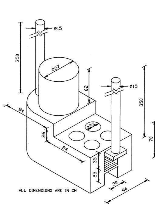
Fig. 3. Traditional cottage basin oven with two chimneys and two rows of cooking basins.
