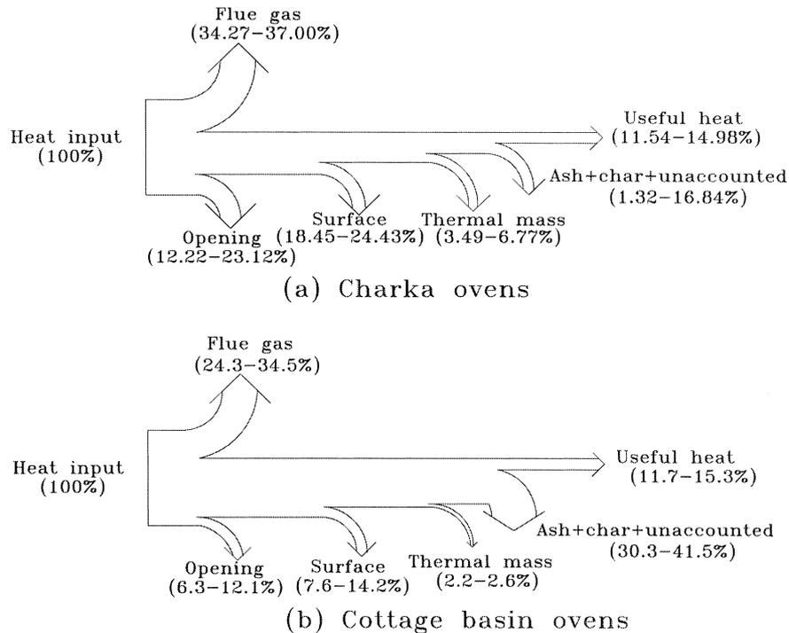
Fig. 7. Sankey diagram showing various heat streams of stoves.
