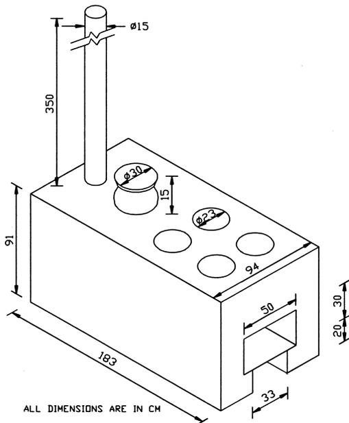
Fig. 5. Traditional cottage basin oven with different size and shape of water preheater.
