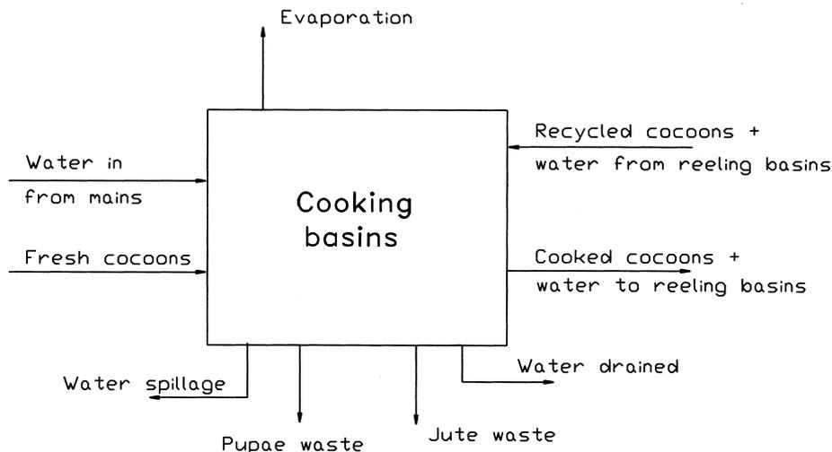
Fig. 6. Water-balance chart for cooking basins.
