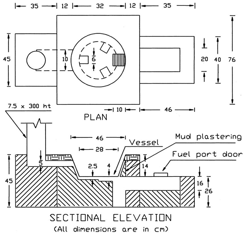
Fig. 1. Technical drawing of a charka oven.
