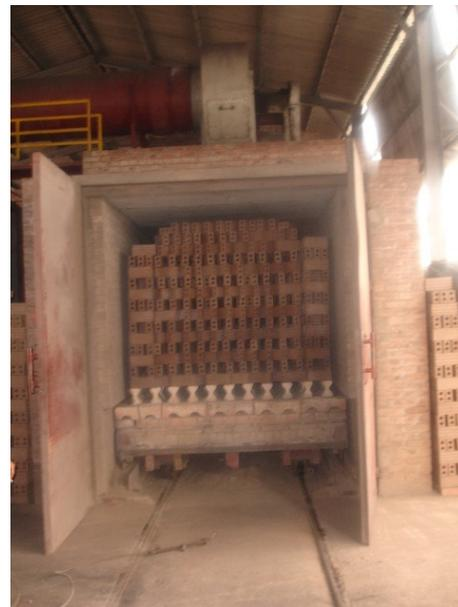
Figure 15 Tunnel kiln for brick firing
