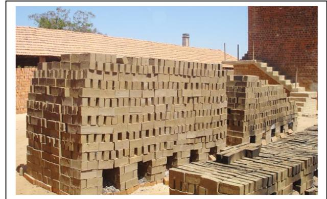
**Figure 9** Artificial stack dryer experimented by an entrepreneur at Malur
