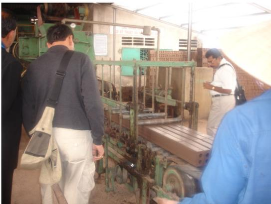
Figure 14 Brick extrusion machines
