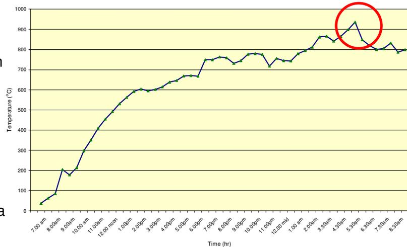
Figure 7 Typical temperature profile in downdraught kiln
