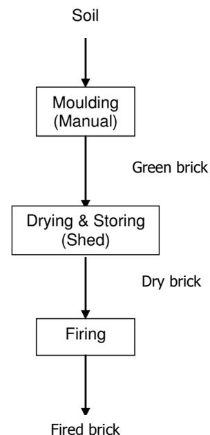
Figure 1 Brick making process
